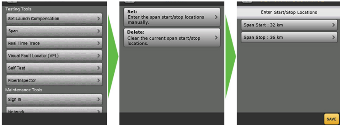
Process to set Span on an OptiFiber Pro OTDR
