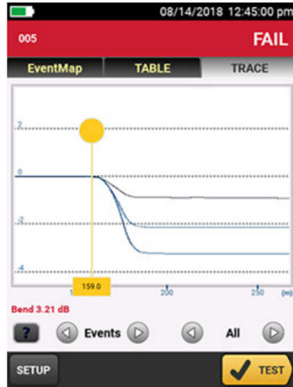
Bend as seen on an OTDR trace
